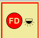
92206 H Space protected by automatic fire alarm
