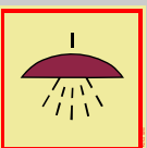
92215-I H space or group of spaces protected by fire- extinguishing system
