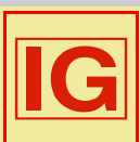
92296 H Inert gas installation
